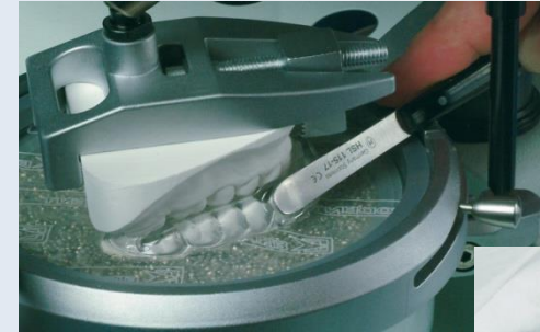
...and immediately press the hot plastic foil material in the cuspid area with a suitable instrument against the antagonistic jaw.
